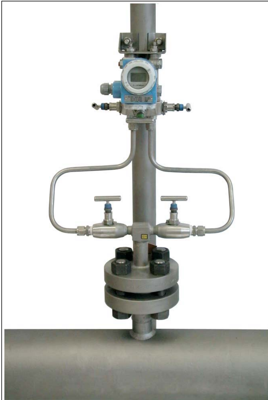
Fig.: 7.2: DP sensor IBF-25 for a pipe with ID 146,3 mm. The DP transmitter is remotely mounted and is connected to the sensor through Ermeto- pipe
