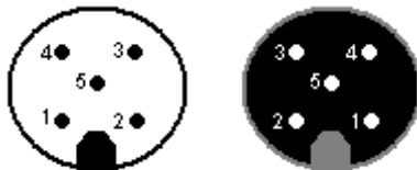
Fig.3: Pin code: Connection plug / socket
