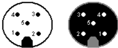
Fig. 7: Pin code: Connection plug / socket for 5-pin version
