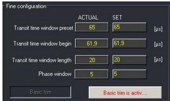
Fig. 23: The status message Basic trim is active in the field Fine configuration
