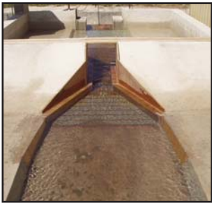
Scale model of a control sluice on a dam on the Huisne
