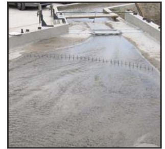
Scale model of a tree trap on the Béoux River (France-05)
