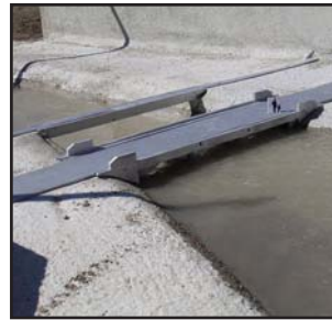
Scale model of a tree trap on the Béoux River (France-05)
