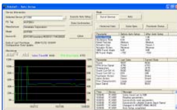
Figure 7 Executing auto setup window
