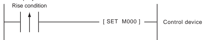
[ Ladder circuit example ]
