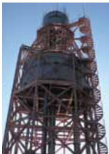
Elevated water tank for flow calibration rig
