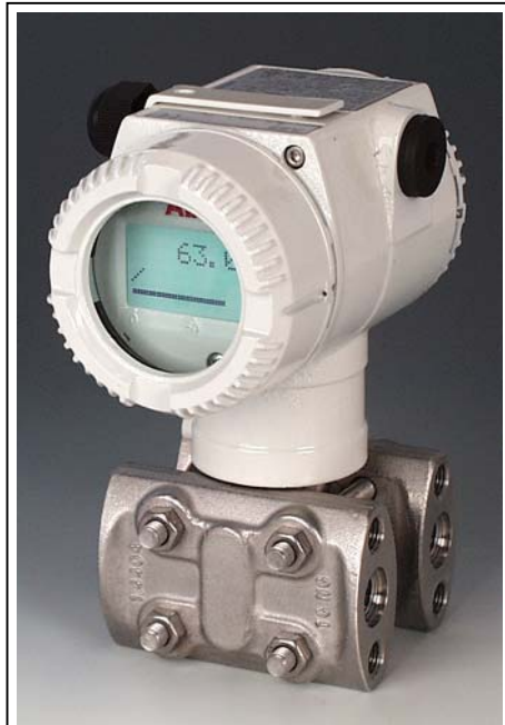
Fig. 1: Transmitter for measurement of volumetric flow, fluid temperature and pressure and calculation of mass flow value
