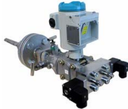
Fig. 3.1: Air purge unit LSP for automatic cleaning of pitot tubes used in gas and gas mixtures containing dust or bubbles
