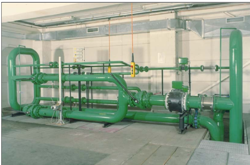
Fig. 12.2: Water calibration test stand for pipe sizes DN 15 (1/2") to DN 300 (12"). Volumetric flow: 0 to 360 m 3 /h (1600 GPM). Temperature: 15 to 25 °C (59 to 77 °F). Pressure: 0.2 – 1.0 bar (2.9 to 14.5 psig).
