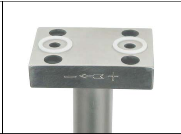
Fig. 7.2: Sensor head with flange plate to direct-mount a 3-way manifold. Limited use w/out pipe insulation, gas to pressure max = 63 bar (914 psig) and temp max = 200 °C (392°F), liquids to pressure max = 63 bar (914 psig) and temp max = 150°C (302°F)
