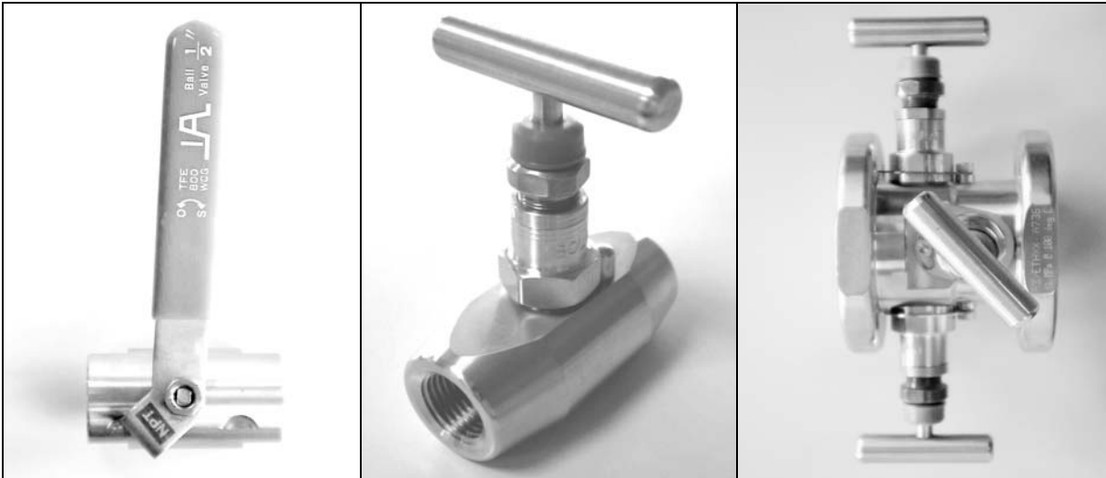
Fig. 7.15: Ball valve PN 40 (580 psi), 1.4401 (316 SS) Fig. 7.16: Shut off valve ½ “ NPT, PN 400 (5801 psi), 1.4401 (316 SS) Fig. 7.17: 3-way-manifold PN 400 (5801 psi), 1.4401 (316 SS)
