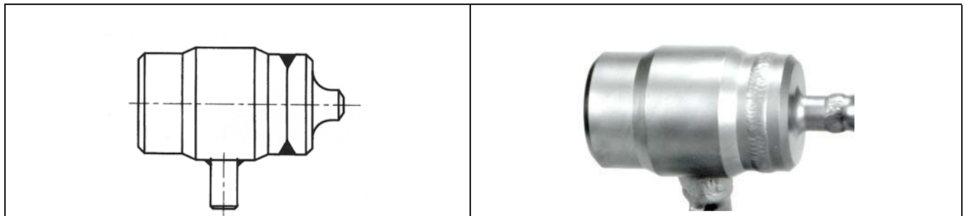
Condensate pots, Dimensions \varnothing 3.54 x 0.69 inches (90 x 17.5 mm) with weld sockets 0.84 inches (21.3 mm)
