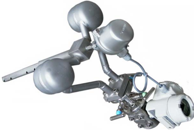
Fig. 8.1: Compact version of a flow sensor used to measure steam mass flow. The components: DP sensor with welded condensate pots, wet-tap temperature sensor, flange plate with 3-way-manifold and DP transmitter to measure the differential pressure, the operating pressure and the operating temperature, and to calculate mass flow.
